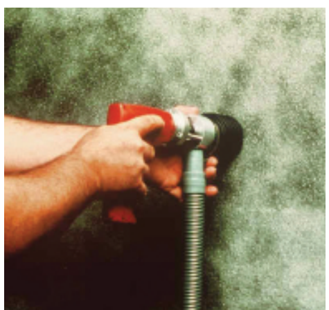
FIGURE 12.19 Needle Gun with HEPA Exhaust Ventilation.
